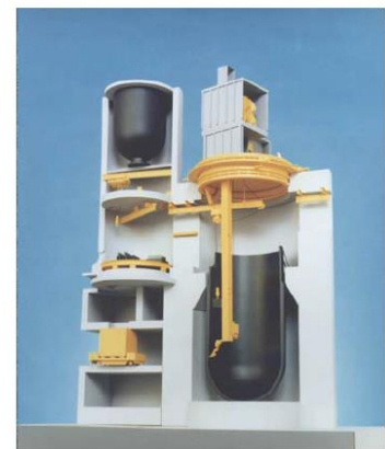
Fig. 6. Decommissioning robot for WAGR reactor [8]
